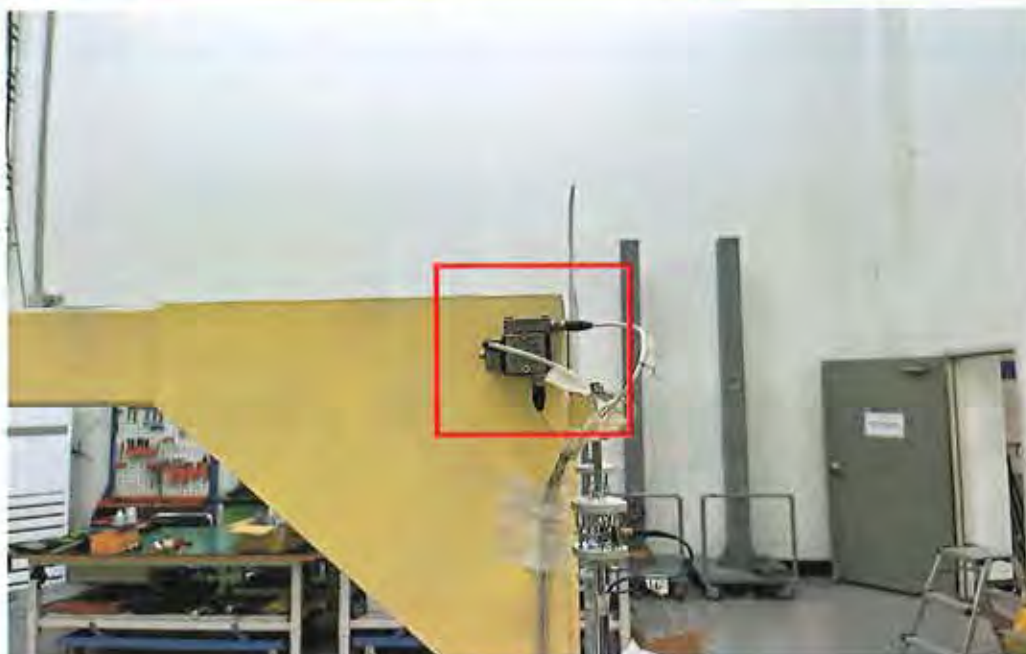
[Figure 4-7] Accelerometer Set up – Fixture
