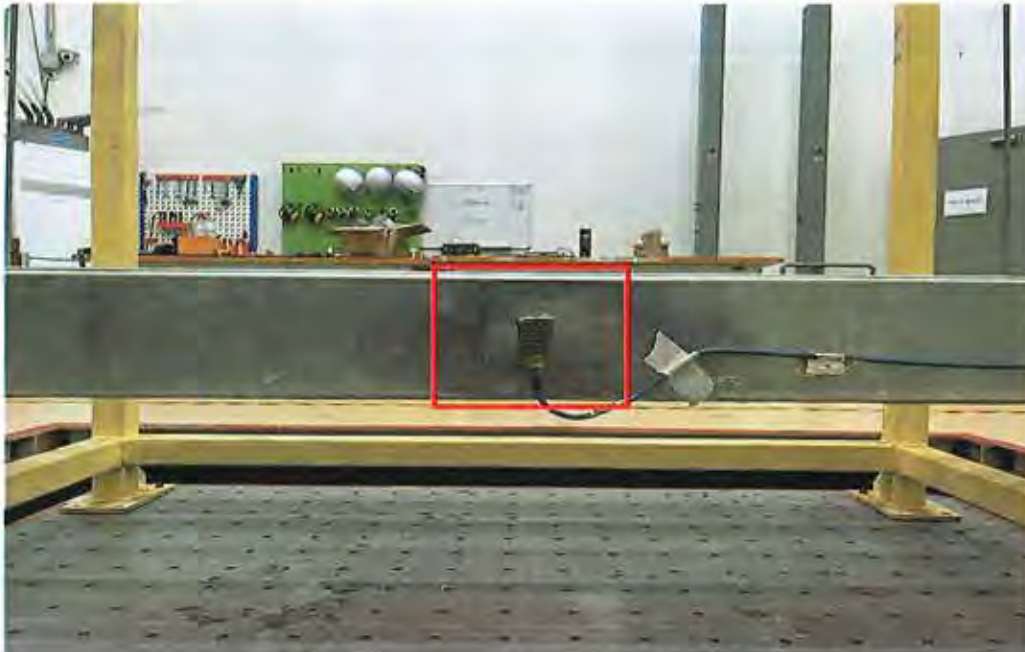
[Figure 4-9] Accelerometer Set up – Cable Tray (1/2)
