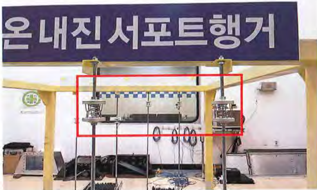
[Figure 1] Seismic Support Hanger – VOS-038-001
