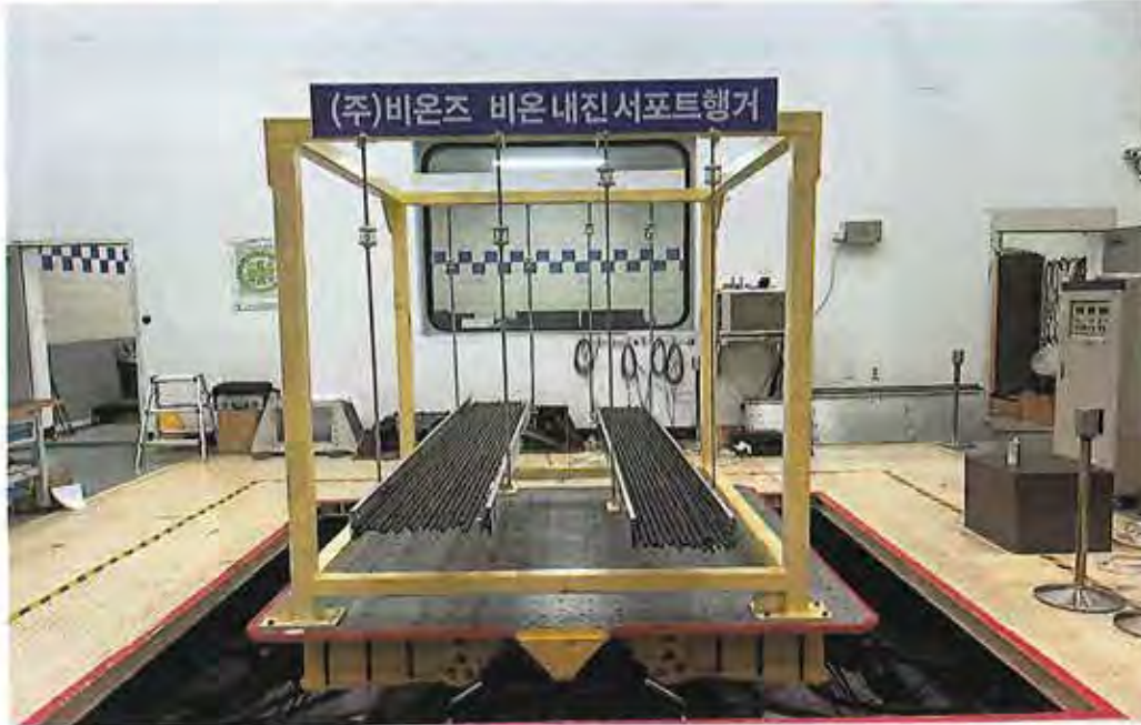
[Figure 4-1] Excitation Test Set up #1
