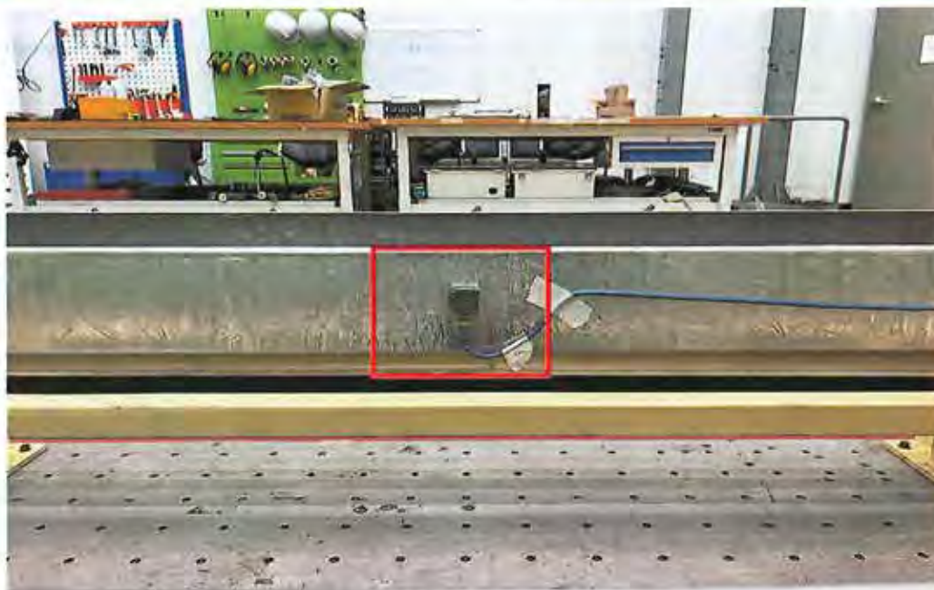
[Figure 4-9] Accelerometer Set up – Cable Tray (1/2)
