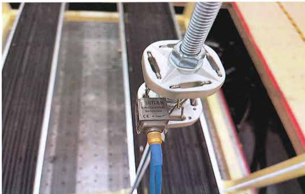
[Figure 4-8] Accelerometer Set up – VOS-012-001
