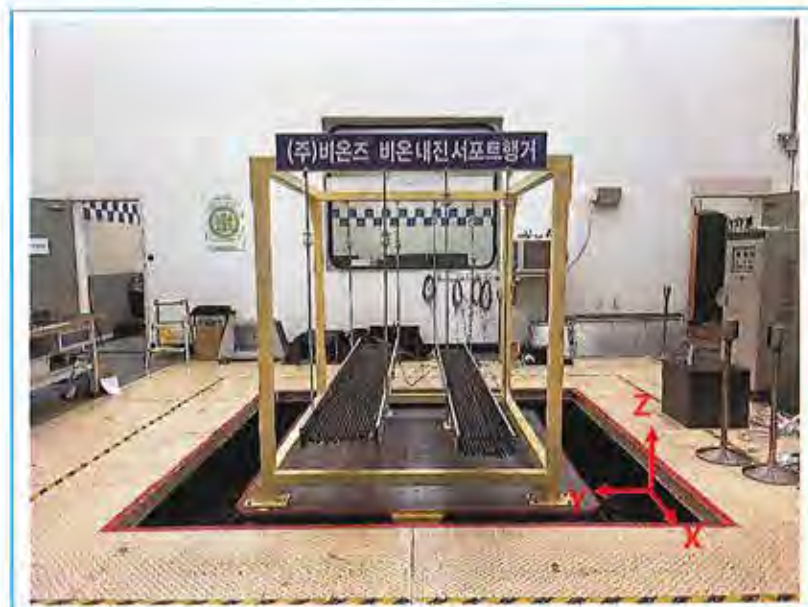
[Figure 3] Seismic Test Setup
